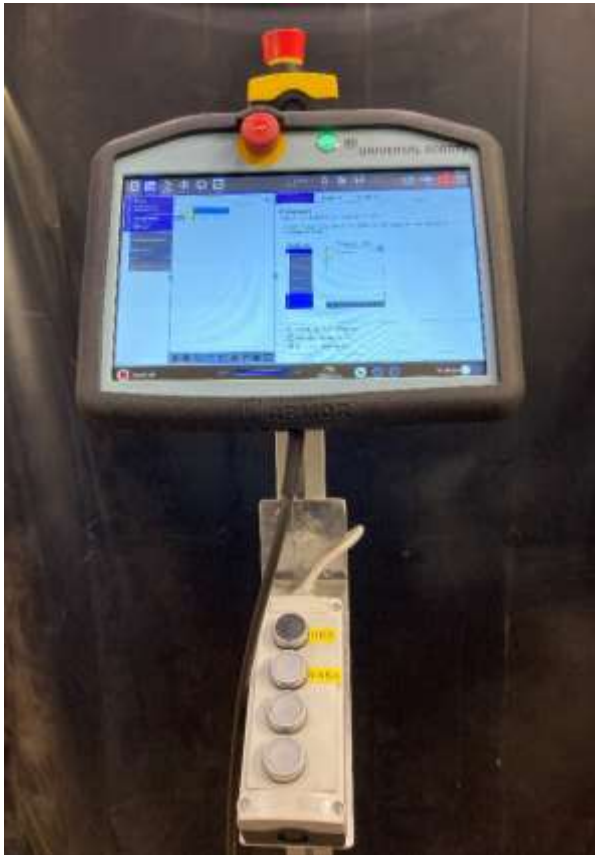
Robot's teach pendant and push buttons
